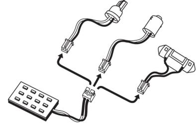
In some vehicles that are equipped with a CANbus control system, the installation of LED bulbs may cause error signals on the dashboard. By using Philips LED warning cancellers, you will avoid those error signals caused by the failure diagnostic of the CANbus system.
