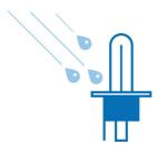
Only a burning bulb made of quartz glass (filament 2650°c, glass 800°c) can resist thermal shocks: such as, if a drop of cold water touches the hot bulb, when you drive through water with a broken headlight unit.
